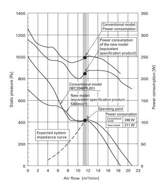
Fig. 7: Air flow vs. static pressure characteristics – Comparison between the conventional model and the equivalent specification model
