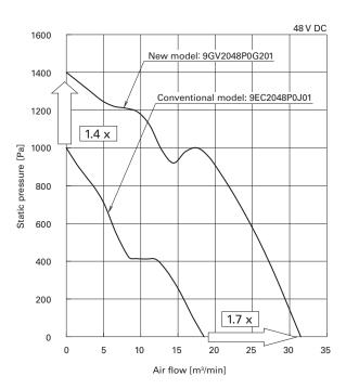
Fig. 5: Air flow vs. static pressure characteristics Comparison between the new model and the conventional model
