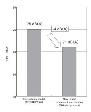
Fig. 9: Comparison of SPL between the conventional and an equivalent specification model
