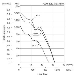
Fig. 3: Air flow vs. static pressure
