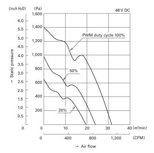
Fig. 4: Air flow vs. static pressure characteristics at individual PWM duty cycle
